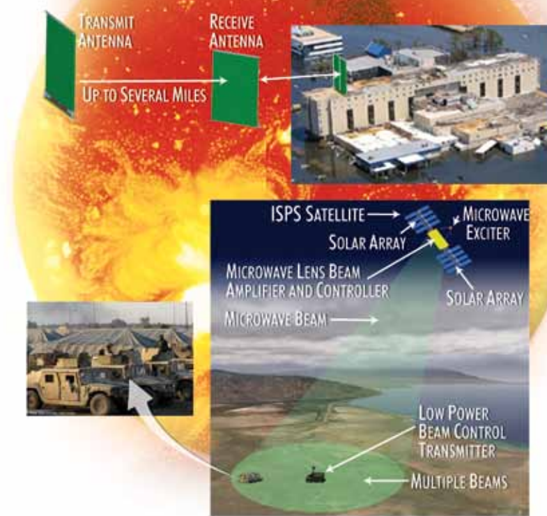
Above: Pictured is an artist's conception of rectennae, erected on the ground, transmitting power to a rectenna installed on the roof of the Methodist Hospital in New Orleans, La., after Hurricane Katrina. Power received is enough to run an emergency operating room.
